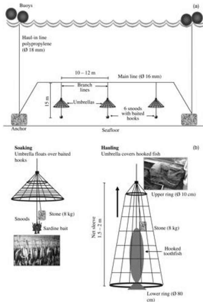
**Figure 3:** Diagram of the ‘umbrella and stones’ physical protection device developed to mitigate sperm whale depredation and seabird bycatch in bottom longline fisheries in the Southwest Atlantic. Figure taken from Goetz et al. (2011).
